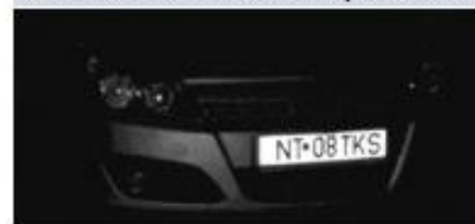
Infrared (IR) illuminator for better number acquisition
