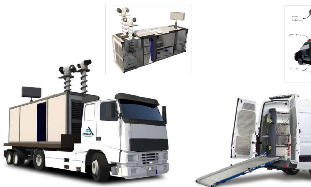
builds customized IED vehicles, that enable the IED team to engage with a suspicious object in an urban area, with minimum risk to public safety. The vehicle may be equipped with a robot, conventional bomb disposal equipment, disruptors, X-ray inspection equipment, searching devices, demolition tools, mine detectors, bomb locators, bomb suits & other specialized IED tools.
